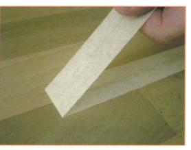
After approx. 10 minutes pull off the masking tape backwards at an angle.
